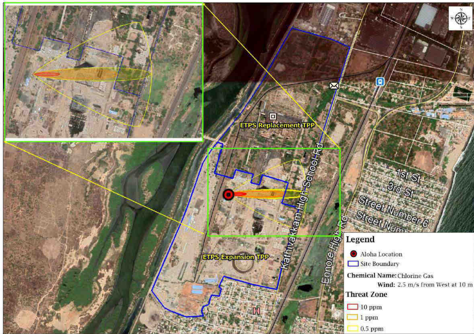
Figure 7.5: ALOHA risk plotting for chlorine gas
